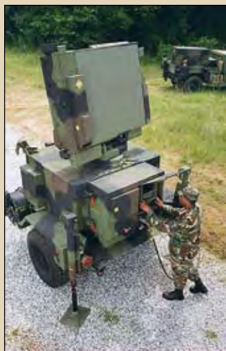
Figure 3 AN/MPQ-64 Sentinel radar is the premier air surveillance and target acquisition and tracking sensor for the U.S. Army's Cruise Missile Defense Systems program.
